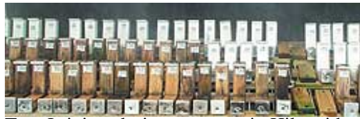
Top: L-joints during exposure in Hilo with differences in mold on paint. Bottom: Greenhouse setup of L-joints for artificial spraying of water.
